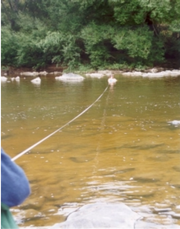
Figure 5.25 Stretching the tape measure across the stream at the start of a cross-section.
