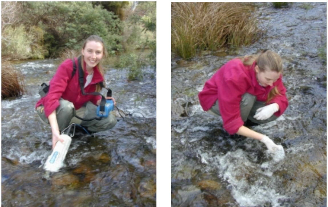
Figure 5.17 Collection of water quality variables using a Hydrolab (left) and collection of a water sample for laboratory analysis (right).
