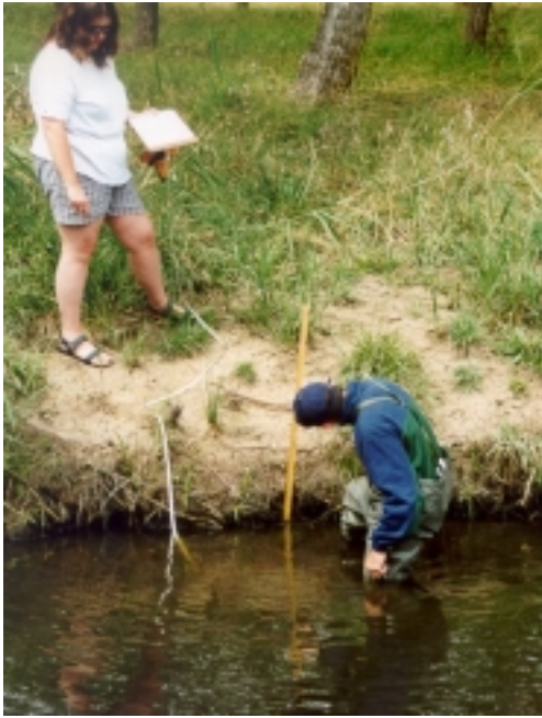
Figure 5.27 Measurement of bank height using a metre ruler or metre ruler and tape measure on a wide bank. In the photo on the right, bank width can also be measured with the tape measure.
