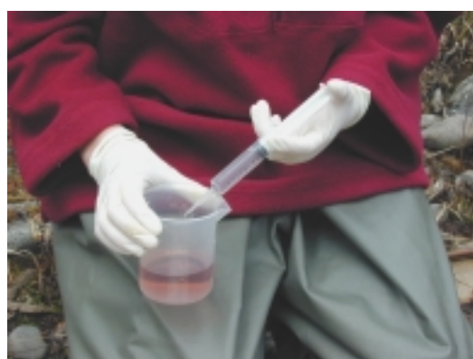
Figure 5.3 Field alkalinity titration. Before addition of acid, the water is green (left) and upon titration endpoint, the water is pink (right).
