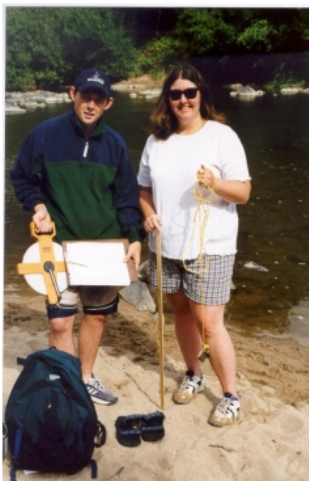
Figure 5.23 Equipment required for measuring cross-sections in a wadeable stream. Note that the metre ruler and weighted rope are interchangeable, depending on stream depth. Waders are not shown because wading shoes were used at this site. Additionally, this photo represents the equipment that needs to be carried to assess the whole of a wadeable sampling site, once water quality measurements have been taken.
